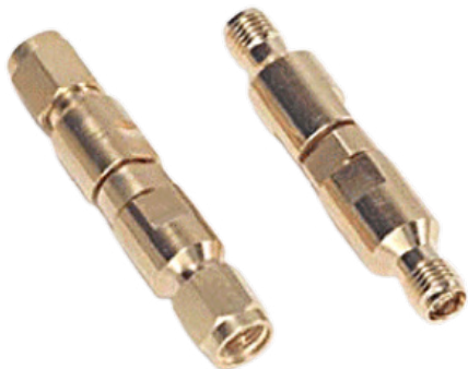
Figure 3. “Connector savers” are coaxial adapters placed between instrument front-panel connectors and cables or DUTs. They can be easily replaced if they are damaged or become worn. Adapters and connectors can be found on www.keysight.com .
