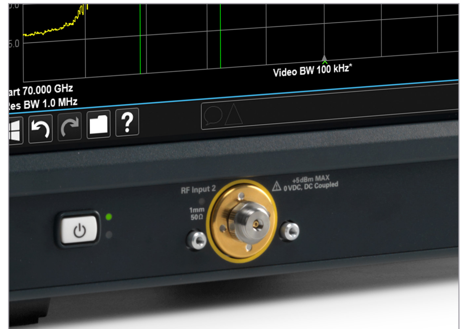
Figure 2. While the typical front-panel connector is female, the gender is often reversed for equipment covering millimeter frequencies (30 GHz to 300 GHz). The male connector offers some degree of protection from several types of damage.
